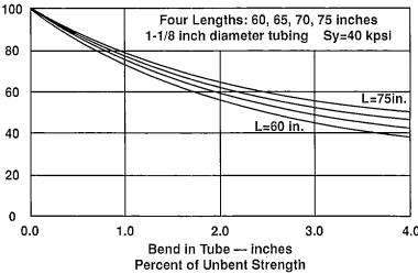
loads (such as bending) applied. We commonly violate these assumptions in two ways: we sometimes apply bending loads (such as during a landing flare) and we sometimes fly with bent tubes. The calculations for failure under either of these conditions is considerably more complicated than under the Euler assumptions. Since our landing flares are close to the ground and at (hopefully!) low airspeeds (and therefore lower loads), those cal-
