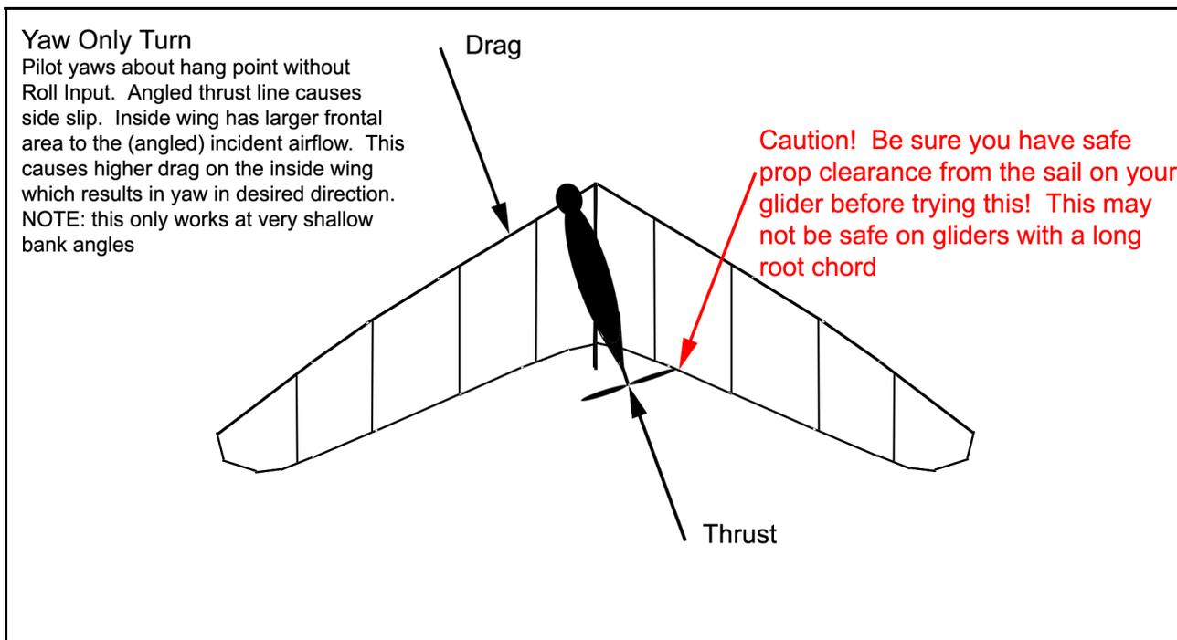
There are definite limitations to the thrust-only turn method - I have only been able to get it to work in smooth conditions and at shallow bank angles. It seems that at steeper bank angles the roll instability of flying under power is too great for this method to overcome. Once I am past more than about 5 or 10 degrees I have to add some roll force to the yawed thrust line in order to reverse the turn.
