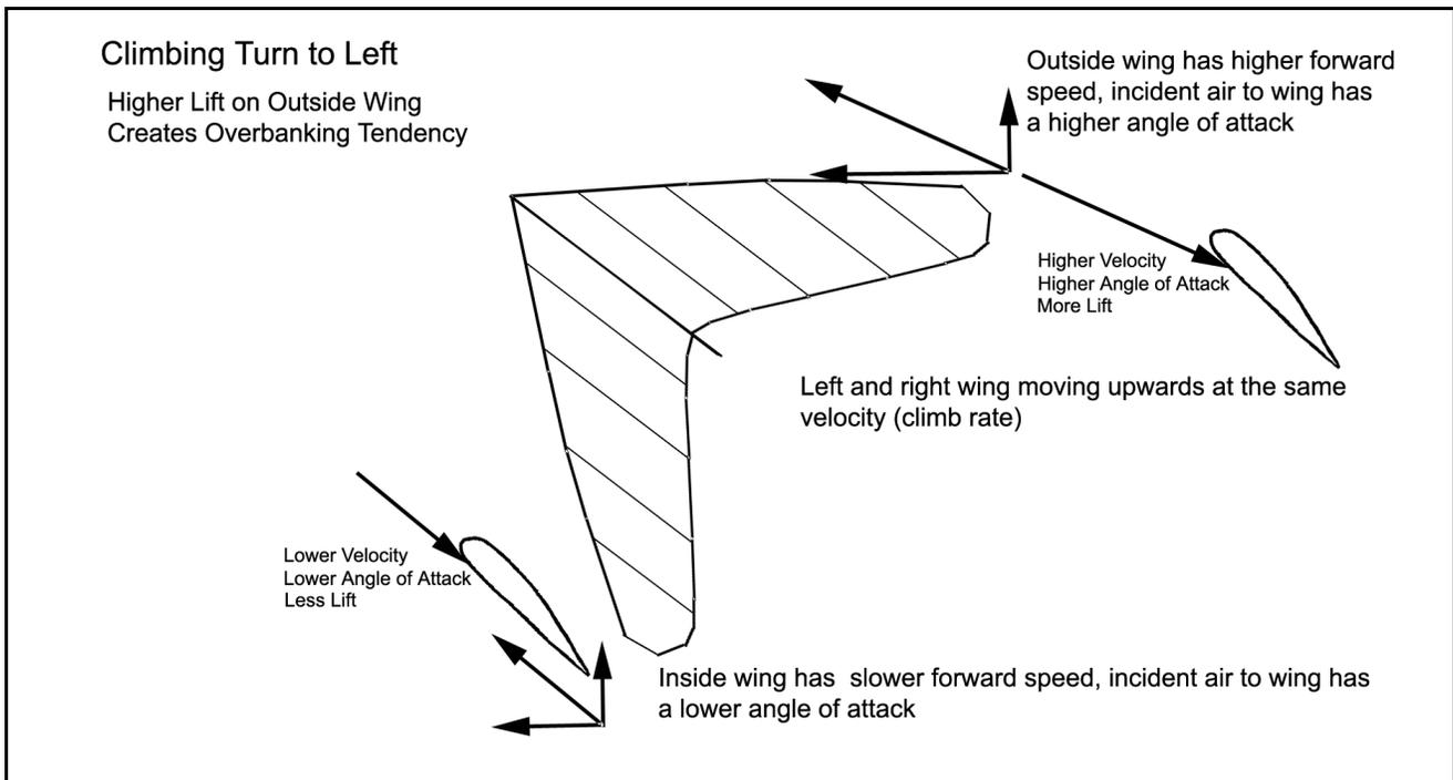
increases for the right/outer wing - so now the right wing has both a higher  $V$  and higher  $C_L(\alpha)$  than the left wing, and the roll moment becomes even larger. Thus we can expect to do more "high siding" to maintain a stable turn under power than we do when gliding.
