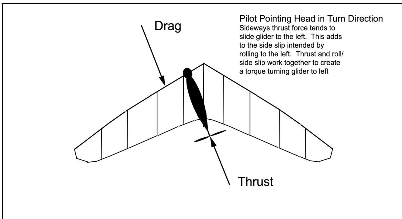
Let's take another look at that, except with thrust added to the picture. The pilot shifts his CG the same amount as with either the parallel or feet-first method, but rotated in the opposite direction from the feet-first method. That is, his head has moved the most to the left and his feet the least. The thrust line now has a sideways component to the left, which is the direction we want to turn and also the
