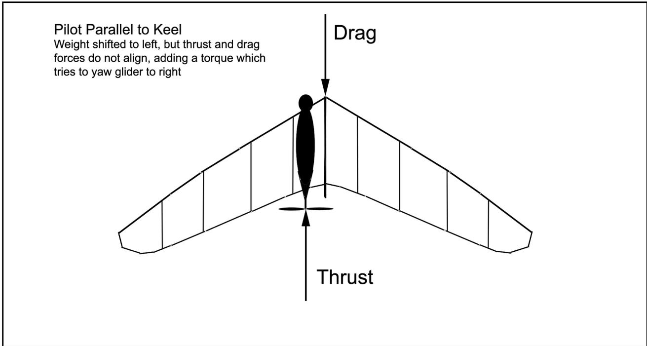
this in a lot of different ways, but the simplest one is to simply think of a twin-engine aircraft with the right engine dead - the thrust acting to the left of the centerline will tend to yaw the glider to the right, just the opposite of what we want.
