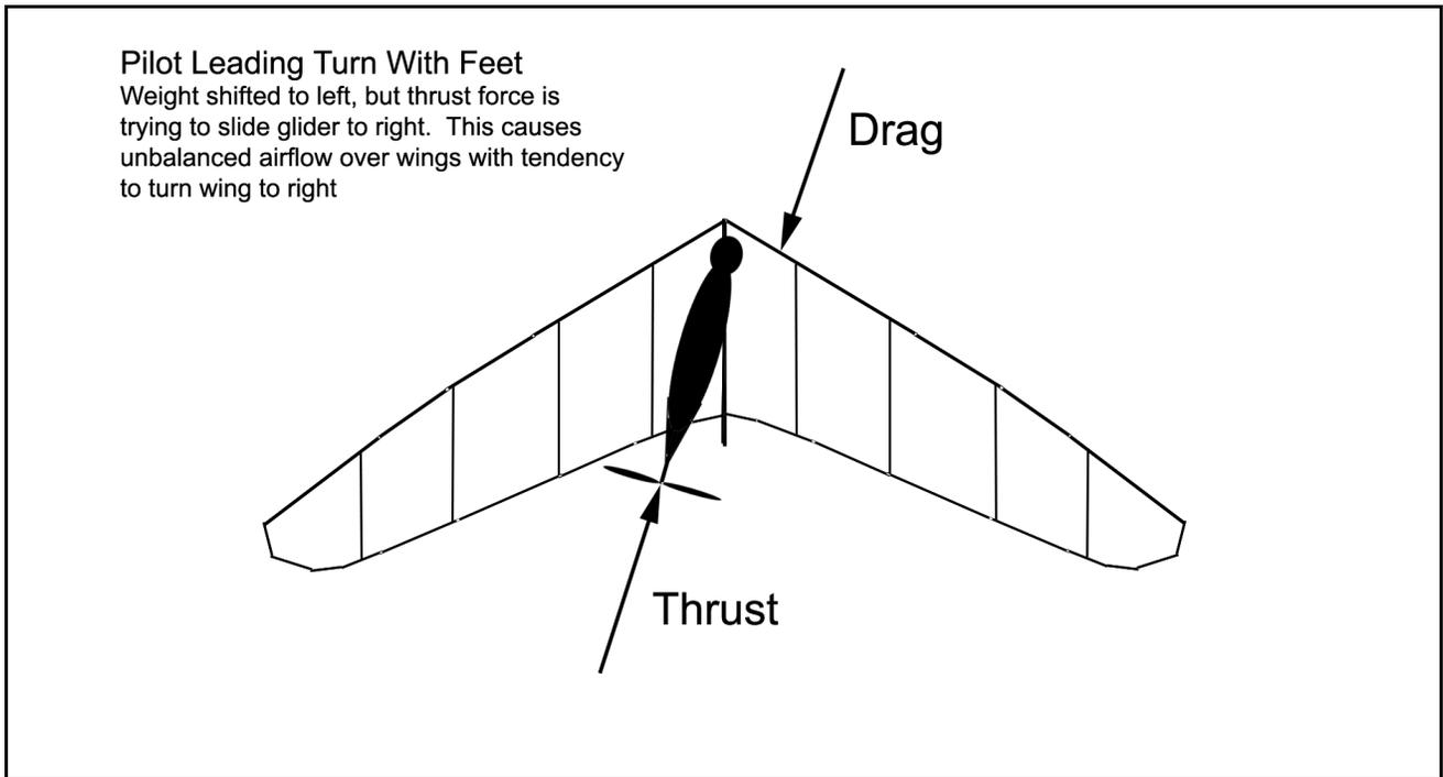
This is the standard method used by many hang glider pilots, myself included (for unpowered flight) -
